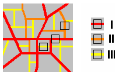
Figure 4. A three level ‘hierarchy’ based on link function. The levels could represent, for example, city roads (I), district roads (II) and local roads (III).
